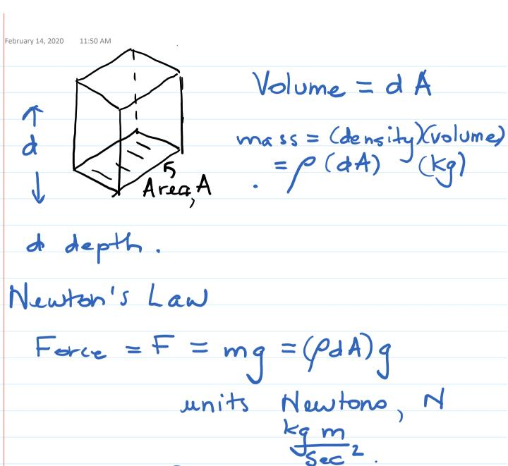
Pressure = P = Force per unit = F/A = pdgUnit Pascals, Pa $kg/m poc^2$ .
